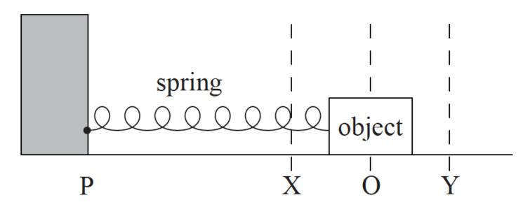
The other end of the spring is attached to a stationary point P. Air resistance is negligible. The equilibrium position is at O. The object is moved to position Y and released.
