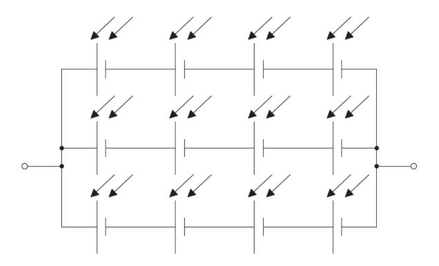
Each cell in the module has an emf of 0.75V and an internal resistance of  $1.8\Omega$ .
