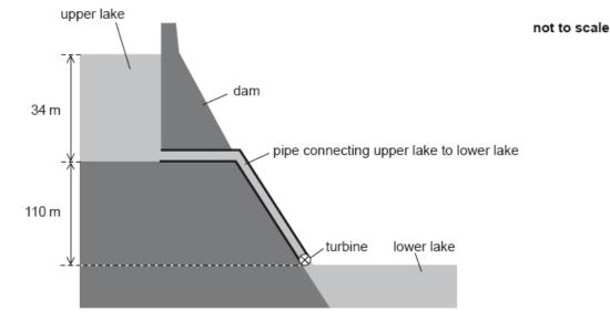
In a pumped storage hydroelectric system, water is stored in a dam of depth 34 m.
